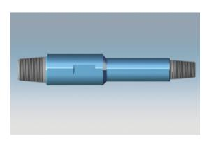
Drill Stem Crossover Subs are short subassemblies used for connecting drill stem components of different thread types or sizes during drilling applications. PPSL Drill Stem Subs are manufactured from alloy steel AISI 4145H Modified, in various OD configurations, in full conformity with API 7-1 specifications & requirements. All connections are machined to API specifications and the thread roots are phosphated in order to minimize galling of threads during the initial make-up.
